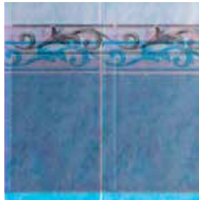
Printing flaws due to irregular belt feed
